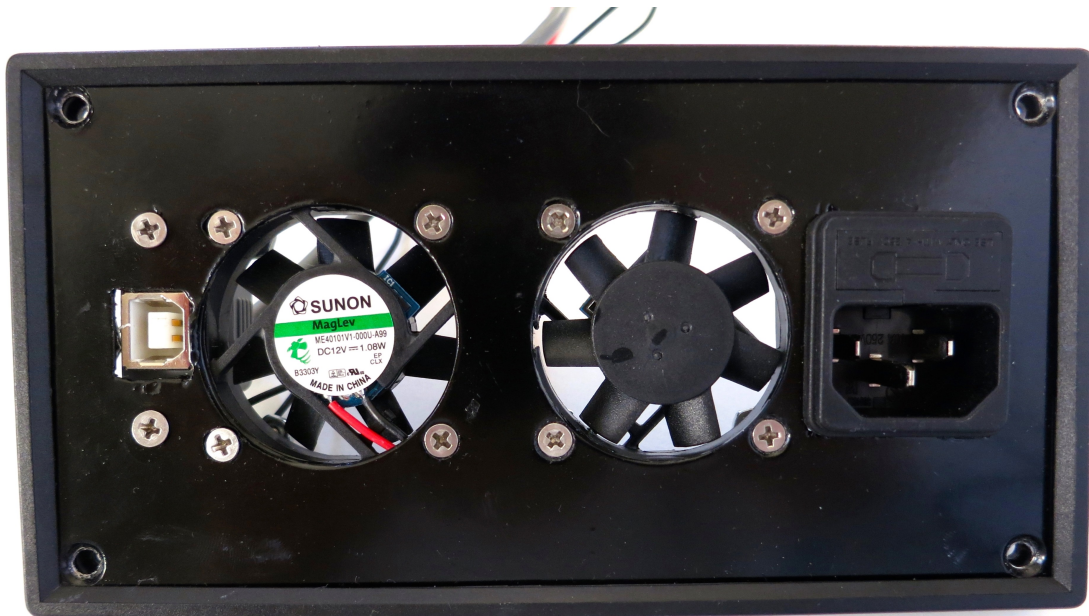
Figure 3.14: The AC to DC converter slotted inside the case.
