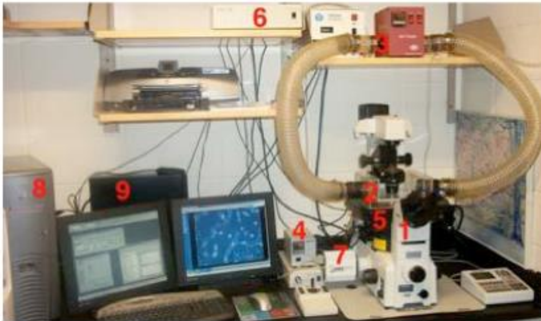
Figure 5. Features of the automated Time-lapse microscopy system.
