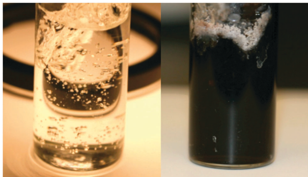
Fig. 3 The initially colorless and optically transparent EDOT gels (left) change to a deep, dark bluish black (right, PEDOT gel) after the UV-initiated polymerization.
